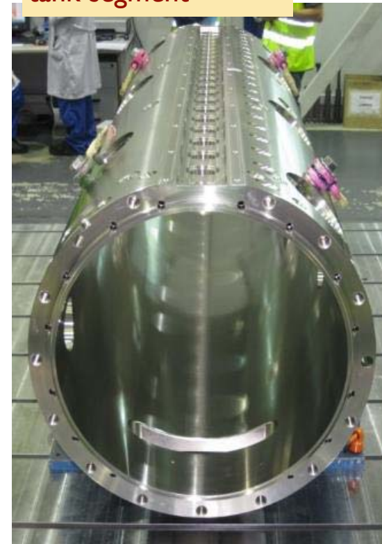
Full scale (~2m) DTL tank segment
