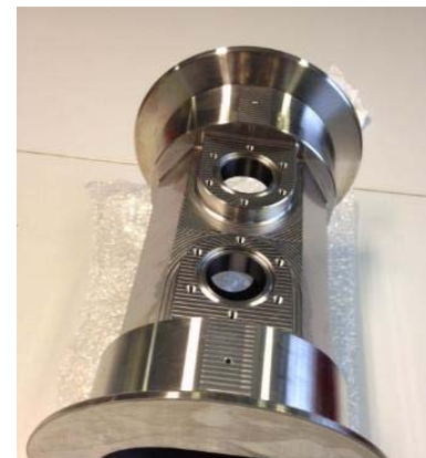
Beam instrument – high-precision machining of 316LN
