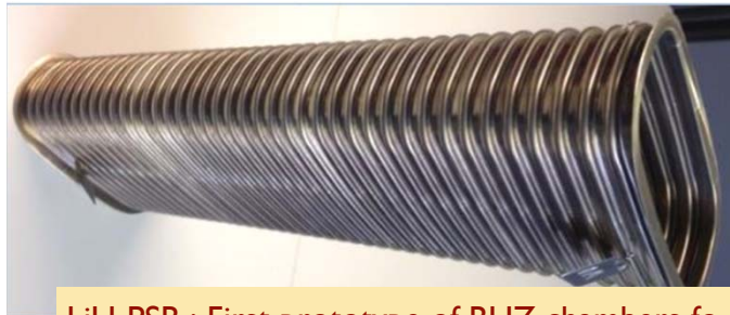
LiU-PSB : First prototype of BHZ chambers for new PSB H- injection (CZ-CH suppliers)
